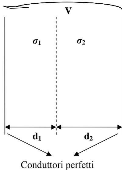
$$\begin{aligned}\sigma_1 &= 2.5 \text{ S/m} \\ \sigma_2 &= 3 \text{ S/m} \\ d_1 &= 0.02 \text{ m} \\ d_2 &= 0.05 \text{ m} \\ S &= 5 \cdot 10^{-4} \text{ m}^2 \\ V &= 2 \text{ V}\end{aligned}$$
