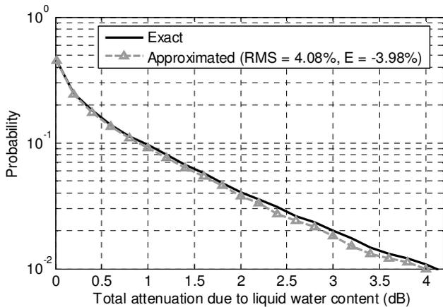
Fig. 4. Zenithal cloud attenuation CCDF at 100 GHz calculated according to the exact (black solid line) and approximate (dashed gray line with triangles) methods for the RAOBS data collected at Milano/Linate airport.
