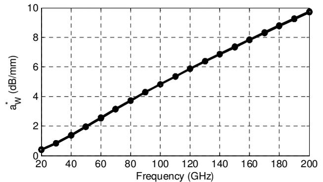
Fig. 2. Trend of the mass absorption coefficient  $a_w^*(f)$  according to (8).
