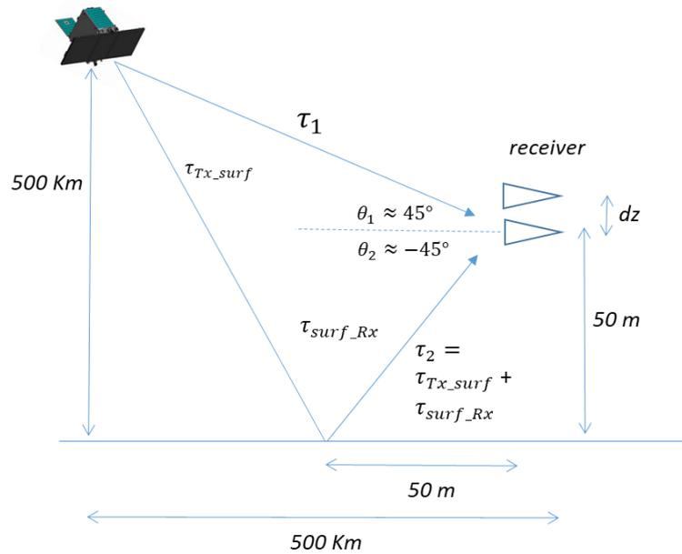
1. Write the expression of the complex envelope of the signals received at the two antennas,  $d_1(t)$  and  $d_2(t)$ . In doing that, make explicit use of the two angles of arrival  $\theta_1$  and  $\theta_2$ . **Tip:** no need for long calculations, just remember the role of the angle of arrival in antenna array theory.
