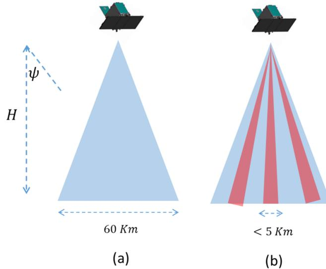
A spaceborne transmitter is equipped with an array of radiating elements to transmit a signal to be received by ground stations. The system operates at a frequency  $f_0 = 5$  GHz at an orbital height  $H = 500$  Km.
