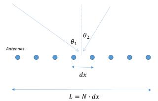
Each antenna is equipped with its own circuity to generate the complex envelope of the received signal.
