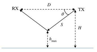
4) Working at  $f = 1.1 f_M = 30.8$  MHz, the wave will be reflected at the ground, so distance *D* can be calculated as:
