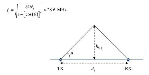
2) The maximum distance  $d_2$  between TX and RX corresponds to the point of maximum reflection along the profile, which corresponds to  $h_{max}$ , i.e. the height where the maximum electron density  $N_{max}$  is found. The maximum distance can be easily calculated as:
