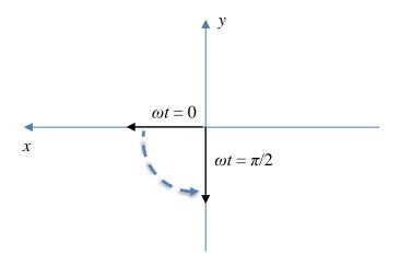
The polarization of the incident wave is LHCP.
