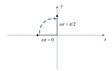
The polarization of the incident wave is RHCP. Note that, as the direction of the reflected plane wave changes (direction = -z), so does also the view of the axes, with the *x*-axis pointing to the right side this time.
